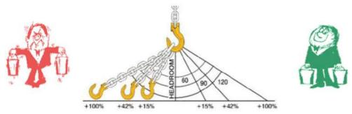
To lift the load with a greater opening angle between the slings, use slings with a higher WLL or reduce the weight of the load
