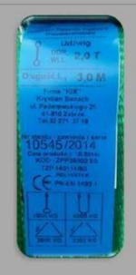
The label of the web sling should be legible and complete. If its damage, illegibility or lack - disqualify the sling from use
