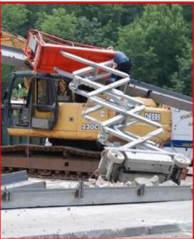
Lifting any materials using platforms (except the necessary tools) is prohibited. Mobile platforms are not transport devices and it is forbidden to use them for this purpose.
