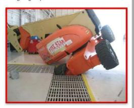
Placing the platform on unstable ground will cause it to tip over. While moving to the workplace or parking place, pay attention to potential obstacles, e.g. sewage wells, unsecured openings or drain gratings and other elements.
