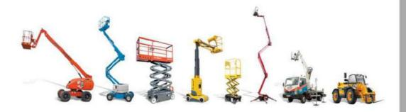
These devices can be powered by electric or internal combustion engines. The use of devices with combustion engines inside halls and rooms is possible only after using exhaust gas neutralizing filters and obtaining the approval of the LG Health and Safety Department.
