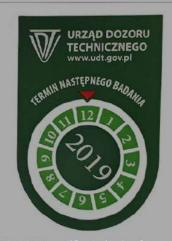
The UDT certificate in the form of a sticker should be placed on the housing of the device in a visible place. (next periodical inspection up to 12.2019)
