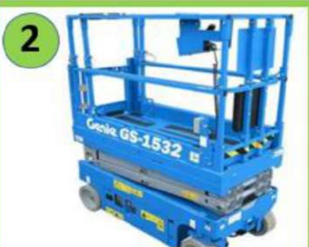
Mobile Elevating Work Platform (MEWP) – PN-EN 280, CE
