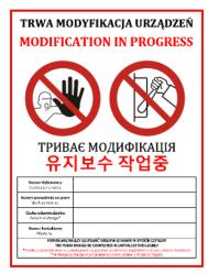
3 Fencing off the work area and marking with the attached label <u>all devices, control</u> <u>panels, cabinets, switchgears, entrances</u> <u>to devices covered by the permit.</u>
